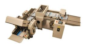
The BAUM 20VFM-1P 1st station module with pile feeder register, and scoring unit can be used with a BAUM CF20 Folder allowing you to do scoring, slitting, perforating and folding heavy weight stock all in one pass. The CF20 can handle heavier weight stocks due to its large diameter fold rolls and gear plate drive for the fold rolls.
