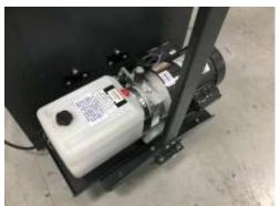
Powerful hydraulic system powers the clamping of the stock AND the knife during the cut.
