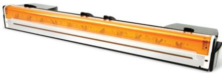
Innovative Memjet® print head has no moving parts and features 70,400 color ink nozzles, providing higher speeds, more precise printing using less ink and producing less noise than standard print heads
