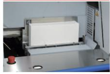
A rigid clamping system holds the book block firmly in position during the milling and nipping process to produce a quality finished book. The safety beam ensures risk-free operation.
