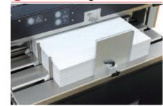
The high capacity cover feed station has a maximum pile height of 150 mm or 5.9" for continuous binding operation. The cover feeder can handle a wide range of covers: Bond Paper 81.4 to 302.4 gsm Coated Paper 104.7 to 348.9 gsm
