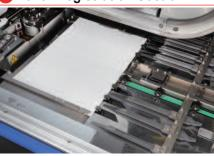
After transport to the nipping section, the cover is registered precisely with the foreedge guide and tail edge positioner.
