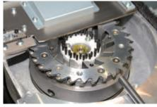
Powerful servo motor driven milling and notching mechanism mills the spine of a book block or signature for optimum glue penetration and adhesion. Milling rotation speed can be adjusted automatically according to book thickness and custom template. Milling depth can be adjusted from 0 to 4 mm or 0" to 0.157".
