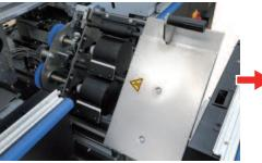
The application drums and back spinner lift and latch to provide easy access for cleaning of the tank.
