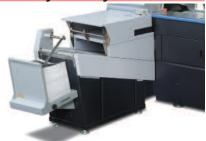
Delivery conveyor to lift the books to a comfortable height for easy off-loading and handlinghandling.
