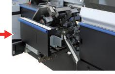
Install the special drain for glue run-off. The PUR tank and drums are teflon coated so that the remaining glue can be easily peeled off after cooling.
