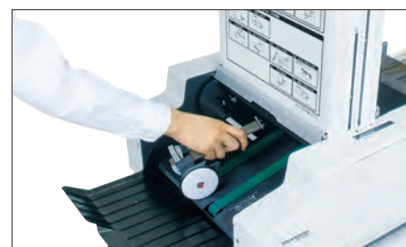
1 Remove the delivery roller.
