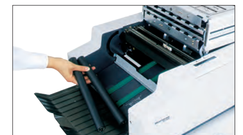
3 Remove the rollers for cleaning or replacement.
