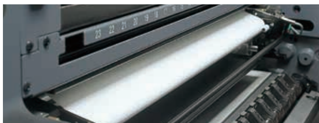
Automatic blanket cleaning device
